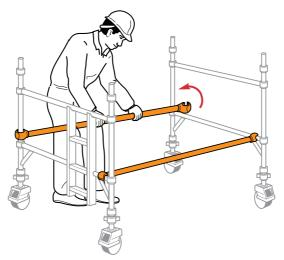
Fit 2 additional end frames ensuring the frame interlock clips are engaged. Fit 2 diagonal braces (blue) in opposing directions, between the 1st and the 3rd rungs. Ensure the frames are vertical and level by checking with a spirit level and setting the adjustable legs as required. Fit stabilisers (see noteson page 30).
