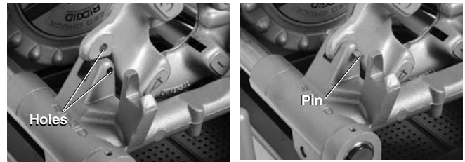
Figure 26 – Retaining LH Die Head in Place
