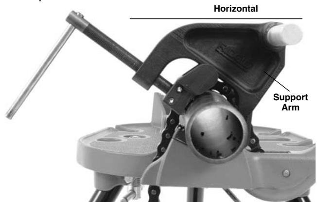
Figure 11A – Positioning the Support Arm
