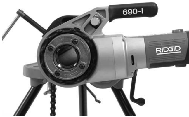
Figure 12 – Proper Orientation of the Power Drive
