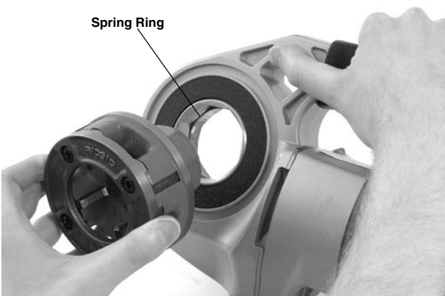
Figure 9 – Installing Die Heads into 600-I Power Drive
