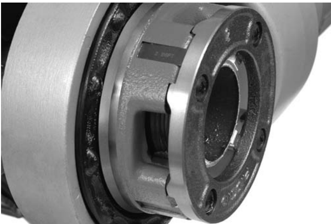
Figure 15 – Pipe Even with Edge of Dies
