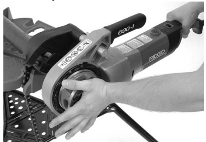
Figure 13 – Starting the Thread
