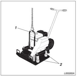
Machine ready for lifting
