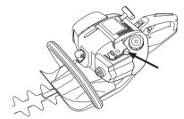
Choke: Set the choke control in the choke position.
