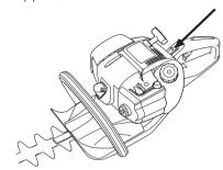
**CAUTION!** The stop switch automatically returns to the start position. In order to prevent unintentional starting, the spark plug cap must be removed from the spark plug when assembling, checking and/or performing maintenance.
