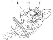
The L and H-jets are used to adjust the supply of fuel to match the rate that air is admitted, which is controlled with the throttle. If they are screwed clockwise the air/fuel ratio becomes leaner (less fuel) and if they are turned anti-clockwise the ratio becomes richer (more fuel). A lean mixture gives a higher engine speed and a rich mixture gives a lower engine speed.
