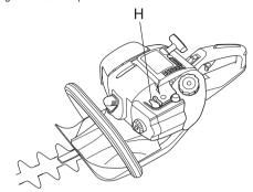
Apply full throttle and turn the high speed jet H very slowly clockwise until the engine slows down. Then turn the high speed jet H very slowly anticlockwise until the engine starts to run unevenly. Now turn the high speed jet H slowly clockwise a little way until the engine runs smoothly.
