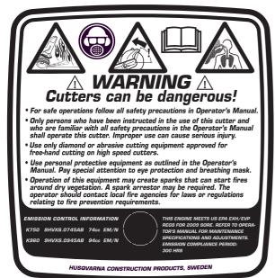
The Emissions Compliance Period referred to on the Emission Compliance label indicates the number of operating hours for which the engine has been shown to meet Federal emissions requirements.
