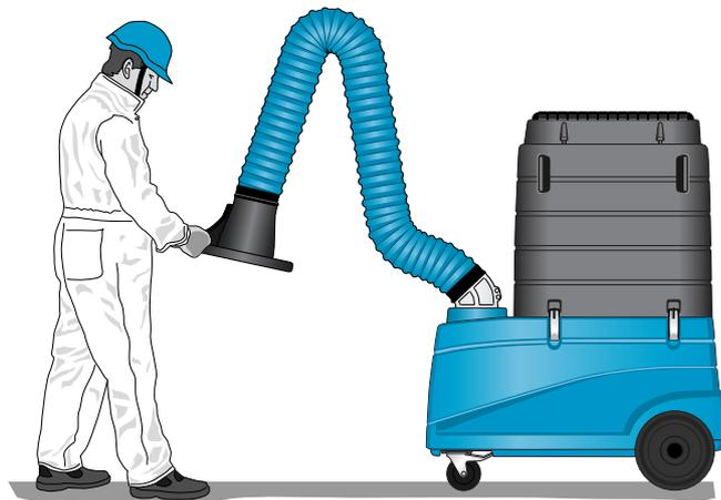
The extraction arm should be positioned with the wheels locked.
