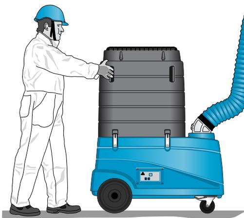
The Filtercart should be moved from behind and with wheels unlocked.
