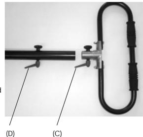
Fix the mains cable at the handle in order to keep it free from the blade and the wheels.
