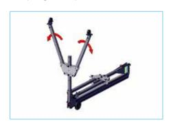
14. Rotate leg assembly around as in steps 8 and 9. Be careful not to trap hands between beam and cheek plates!
