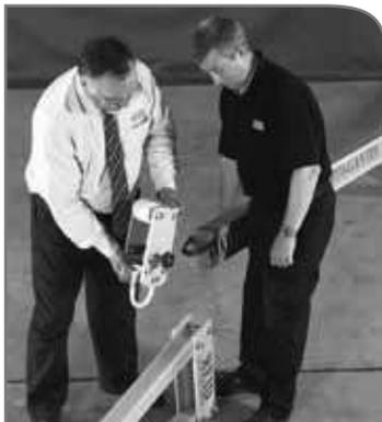
Thread beam trolley over the other end of the beam and lock with friction brake at approximately centre position.
