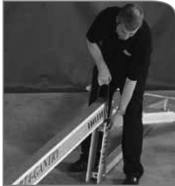
Offer one end of the beam to the rear bolt-hole on the cheek-plate (Bolt 1) and insert a bolt. Put on plain & spring washers and nut, finger tight.
