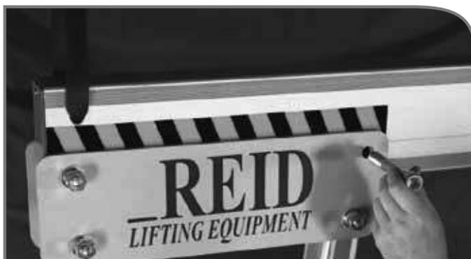
Insert and tighten the final beam bolt.
