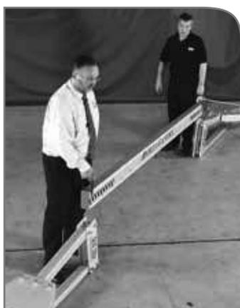
Lay the two A-Frames a beam length apart on a flat surface in line with each other with the castor wheels outward and brakes on.
