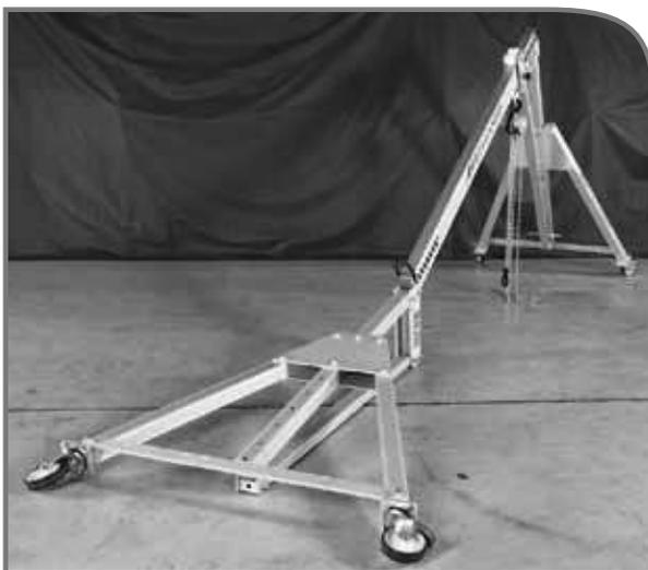
Move trolley to other end of beam, opposite to the end to be raised, and secure by tightening the trolley knob.
