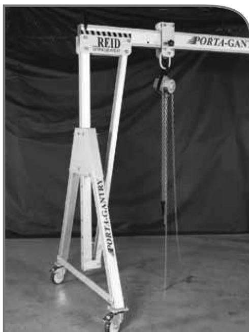
If the hoist is not already attached to the suspension point on the trolley, do so now (using stepladder if height setting requires).
