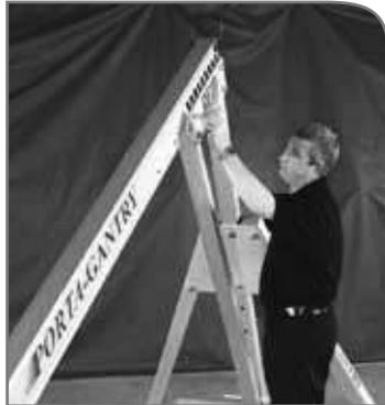
Insert the second bolt into the cheek-plate. Tighten both bolts. (Do not over tighten)
