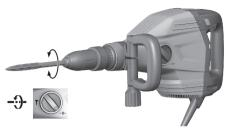
► Set the function selector switch to -9 and position the chisel as desired.
