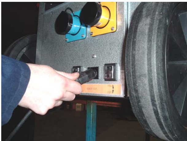
Plug the remote stat lead into the remote stat socket.
