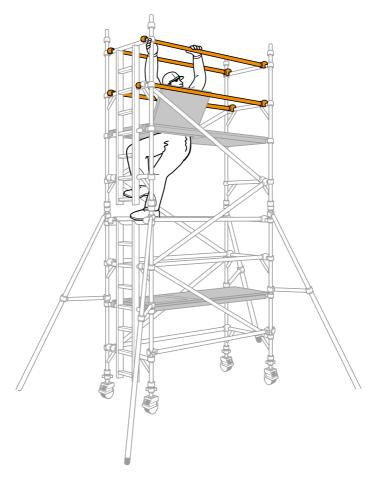
6 Continue the procedure until the required working height is reached, adding additional pairs of end frames, diagonal braces and fitting trapdoor platforms, as shown on previous steps. At every platform level, add horizontal braces as guardrails from the protected position within the trapdoor (as shown in **Step 5**).
