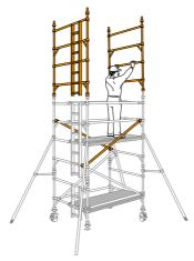
Add two more diagonal braces between the 5th and 7th rungs. If finishing at this height (4.2m platform) reposition the fixed deck to the 8th rung on the tower. Fit a trapdoor deck alongside it, with the hinges towards the outside of the tower, and the trapdoor next to the ladder. Add a single diagonal between the 7th and 9th rungs as shown. Climb up the ladder, and from the protected trapdoor position, fit the guardrails on the 9th and 10th rungs, in that order, on both sides of the tower.
