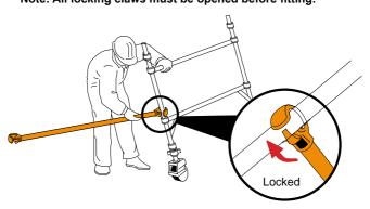
**3** Position the ladder frame as shown and fit the other end of the horizontal brace on to the vertical (just above the bottom rung). Fit a second horizontal brace between the bottom rungs on the other side of the frames to square the tower.
