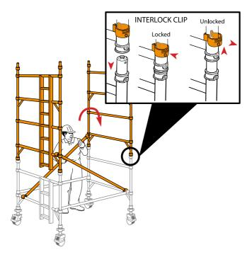
**5** Fit a temporary deck on the lowest rungs. Fit a trapdoor deck on the 4th rung (2.0m) with the trapdoor next to the ladder. Ensure the trapdoor is positioned with the hinges towards the outside of the tower as shown. Climb the ladder and, from the protected trapdoor position, fit guardrails on the 5th and 6th rungs (in that order) on both sides of the platform.
