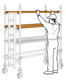
**3** Fit two diagonal braces in opposing directions between the 1st and 3rd rungs. Ensure that the frames are vertical and level by checking with a spirit level and setting the adjustable legs as necessary. Fit stabilisers (see notes on **page 30**). Fit the next pair of end frames and check the frame interlock clips are engaged.
