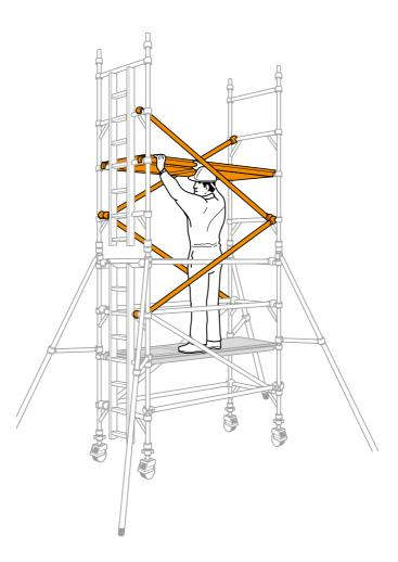
**5** Climb up the inside of the tower and from the protected position of the trapdoor, fit guardrails to the 7th and 8th rungs (in that order) on both sides of the tower.
