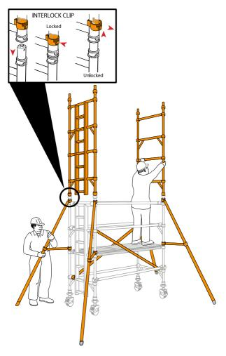
**4** Fit two pairs of diagonal braces in opposing directions between the 3rd and 5th rungs and the 5th and 7th rungs. Locate a trapdoor deck on the 6th rung, with the trapdoor next to the ladder.
