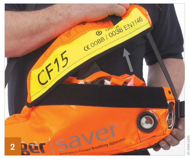
Grip the loop on the lid of the carrying bag and pull firmly upward to break the anti-tamper tag. Open the flap of the bag which then releases the locking clip from the valve turning on the air supply to the hood.
