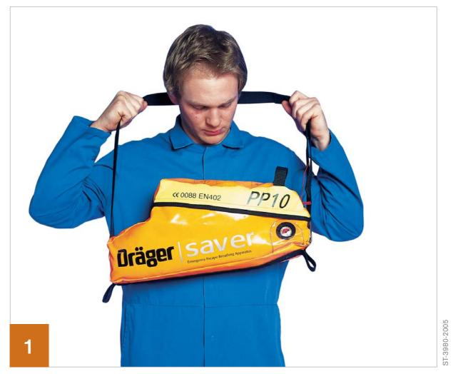
Place neck strap of carrying bag over head. Adjust length of strap until equipment sits in the centre of chest. Fix waistbelt, if fitted, and adjust by pulling the free end until equipment is secure and comfortable.
