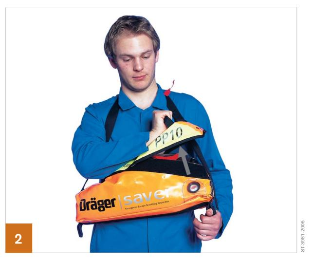
Grip the loop on the lid of the carrying bag and pull firmly upward to break the anti-tamper tag. Open the flap of the bag which then releases the locking clip from the valve turning on the air supply to the head.
