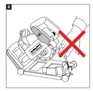
**Caution!** Pull the plug out of the mains socket carrying out any work on the machine. Make sure that the diamond discs are not damaged in any way i. e. no cracks or broken segments.
