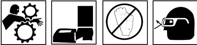
**Do not wear gloves or loose clothing when operating Power Drive. Keep sleeves and jackets buttoned. Do not reach across the machine or pipe.**
