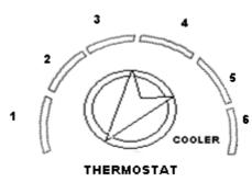
The compressor is controlled by a thermostat which senses the return air temperature. This thermostat can be set to approximate temperatures by means of the thermostat dial, located below the control switch.
