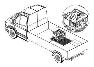
During transport make sure the power pack is secured. Ensure that the power pack is upright during transportation and lifted with approved lifting equipment.
