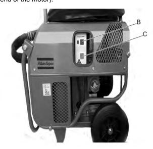
4. If the motor rotates in the wrong direction, stop the motor immediately. Disconnect the electric socket and switch the phases by turning the two pins in the electric socket. Reconnect and start the motor again.
