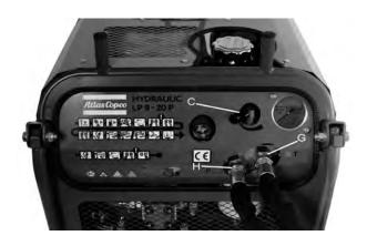
The by-pass valve (C) must be in the OFF position when starting and in the ON position when using the machine.
