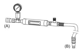
To set or check the hydraulic oil flow and the pressure relief valve we recommend using Atlas Copco or similar test equipment.
