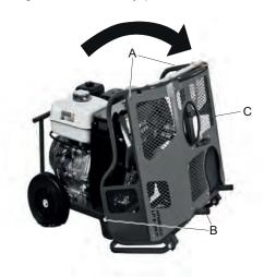
Remove the screws (A) and loosen the screws (B), in order to open the cover (C).
