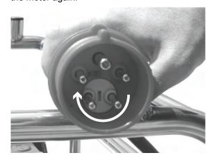
*NOTICE* Letting the motor rotate in the wrong direction for a long time can harm the pump.
