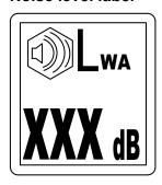
The label indicates the guaranteed noise level corresponding to EC-directive 2000/14/EC. See "Technical data" for accurate noise level.
