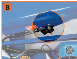
A. Powerpack Emergency Lowering Valve (undercover)
