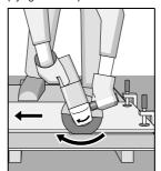
The machine must always work in an upgrinding motion. Otherwise, the danger exists of it being pushed uncontrolled out of the
