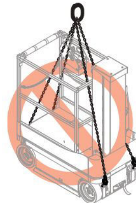
Figure 3-11. Inappropriate Lifting Method
