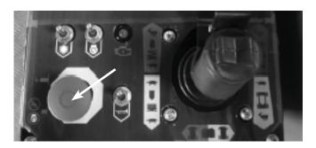
Figure 9.1 - Platform Control Box Emergency Stop Switch
