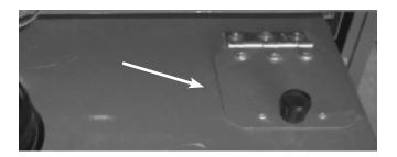
Figure 7.7 - Radiator Cap Access Hatch
