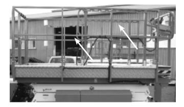
Figure 7.20 - Primary Fall Restraint System
