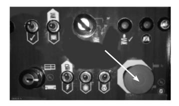
Figure 8.1 - Emergency Stop Switch at Ground Control Box
