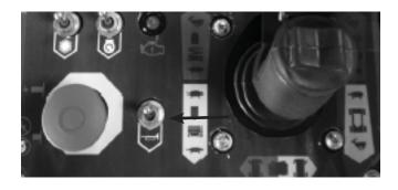
Figure 2.10 - Operator Horn
