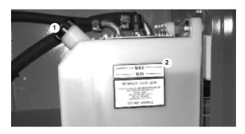
Figure 7.13 - Hydraulic Oil Tank
