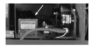
Figure 11.6 - On-Board Battery Charger
