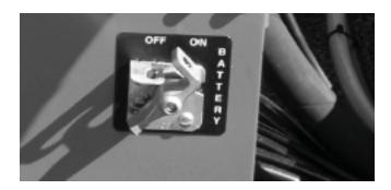
Figure 6.2 - Battery Switch
