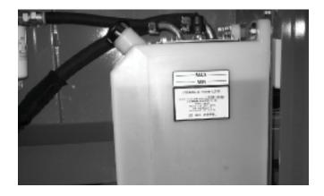
Figure 4.4 - Hydraulic Oil Level
