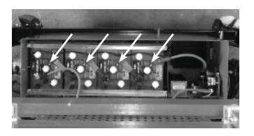
Figure 11.5 - DC Motor Batteries
