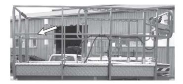
Figure 2.5 - Fall Restraint
