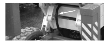
Figure 7.11 - Wiring Harness in the Scissor Stack
