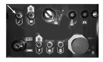
Figure 2.12 - Enable Switch
