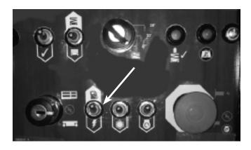
Figure 11.2 - Diesel / Electric Selection Switch
