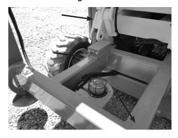
Figure 7.19 - Structural Damage and Welds
