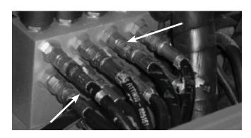
Figure 7.14 - Check Fittings at Valve
