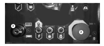
2. At the ground control box set the emergency stop switch (2) to off, turn the main power switch (3) off and remove the key (see figure 9.8).
