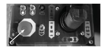
Figure 8.2 - Emergency Stop switch at Platform Control Box
