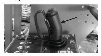
Figure 2.8 - Joystick Safety Control
