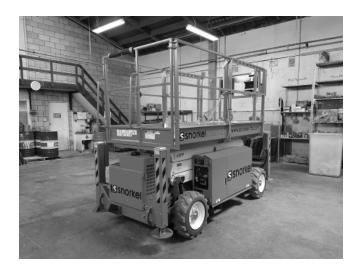
Figure 10.1 - Correct Stowed Position
