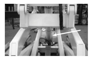
Figure 7.15 - Check Hydraulic Cylinders
