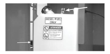
Figure 7.3 - Fuel Leaks at Tank
