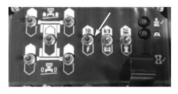
Figure 11.4 - Fuel Switch, Platform
