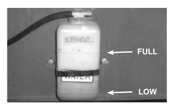
Figure 7.6 - Engine Coolant Level
