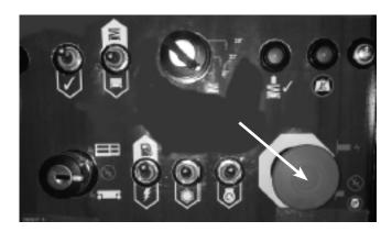
Figure 9.2 - Ground Control Box Emergency
